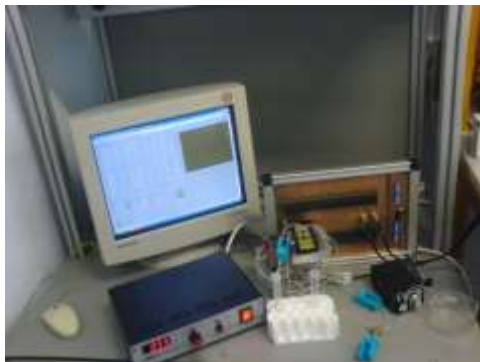
Fig. 5: In order to perform the oligo experiments tight control over the sample temperature is required. Therefore the hybridization cassette was allowed to settle on a hotplate whose temperature could be regulated to within 0.1°C. Furthermore, in order to minimize bubble formation manual pinch valves were introduced in the fluidic circuit thus increasing the control over the flow of the various fluids. Fluid control was achieved using a peristaltic pump at the exit of the fluidic circuit. Finally a relay matrix undertakes the task of switching each sensor in the array to a capacitance meter.
