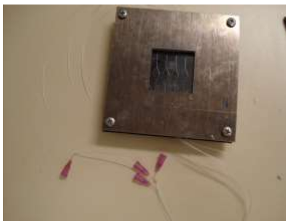
Fig. 1: Aluminum plates with a light window enclosing the patterned PDMS gasket with the four independent fluidic channels. Also shown are the four fluidic inlets.
