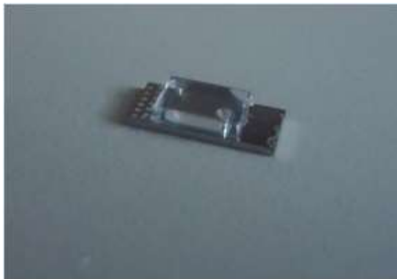
Fig. 3: Functionalized Fully Integrated PYTHIA chip (9.26X4.00mm 2 ) with the flow cell on top
