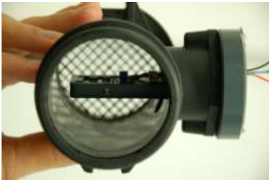
Fig. (a): View of the interior of the automobile engine inlet tube with the air flow meter mounted in it.
