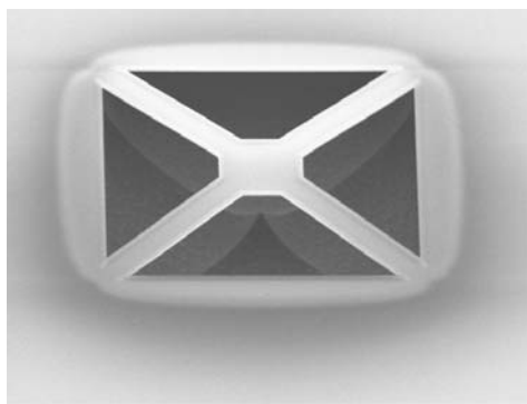
Fig. III.1.6: Fully released porous silicon micro-hotplate used as test structure for the stress measurement. The thickness of the membrane is 4 μm.
