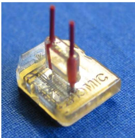
**Fig. III.2.3:** Packaged device, with all electronic and fluidic connection in place, for use in the field in a portable instrument.
