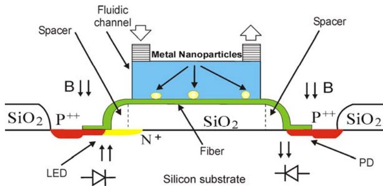
**Fig. III.2.1:** Schematic illustration showing the monolithic optoelectronic bio-transducer coupled to a fluidic module. This fluidic module is shown below and covers in series all nine fibers per chip.
