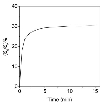
**Fig.III.2.4:** Real-time response plotted as the ratio of the initial detector photocurrent ( $S_0$ ) to the instantaneous photocurrent ( $S_1$ ). The CK-MB concentration 300 ng/mL.
