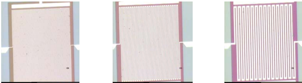
Fig. I.4.3: Gas sensors formed by depositing the heating element on a patterned SnO 2 film. The heating elements have line widths of 2 (left), 4 (center) and 6 μm (right).
