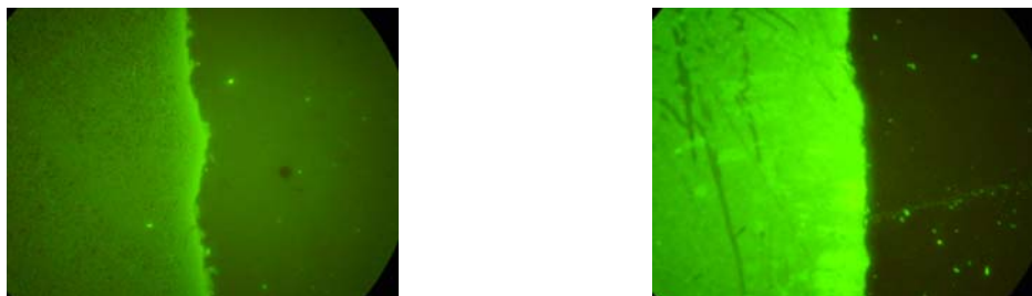
Fig. I.4.6: Adsorption of RgG on colored (left) and bleached (right) WO 3 strips. For the colored strips the photoluminescence intensity is almost equal on the strip and on the glass substrate (left photo). The photoluminescence intensity on the bleached strips is much higher than on the glass (right photo).
