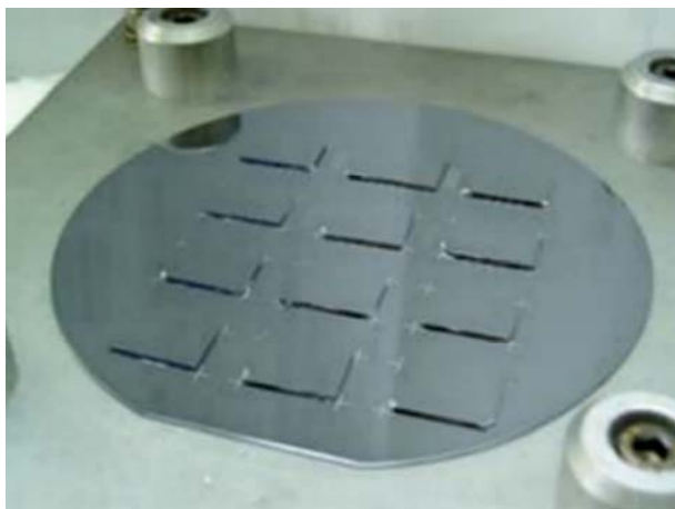
Fig. III.5.3: Four-inch wafer with multiple dies bonded on specific regions.
