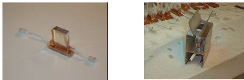
Fig. I.4.8: (Left) Photo of an encapsulated concentration solar cell. A prism ensuring the even distribution of energy on its surface and the current leads are integrated on the encapsulation. (Right) Photo of a cell ready to be positioned on PROTEAS.
