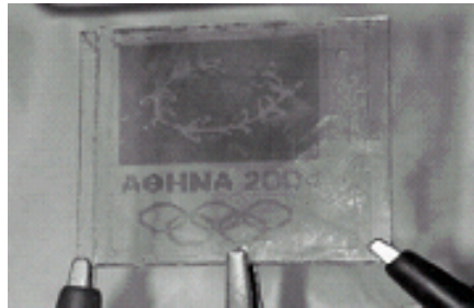
Fig. I.4.7: An all solid-state electrochromic display
