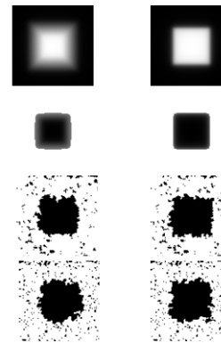
Fig. 2. Grafted and linear chains with 20 monomers / chain, Monomer radius= 0.5nm. Holes nominal CD= 45nm. EDF is determined from 3D Monte Carlo simulation and with convolution with the trapezoidal or the rectangular function.
