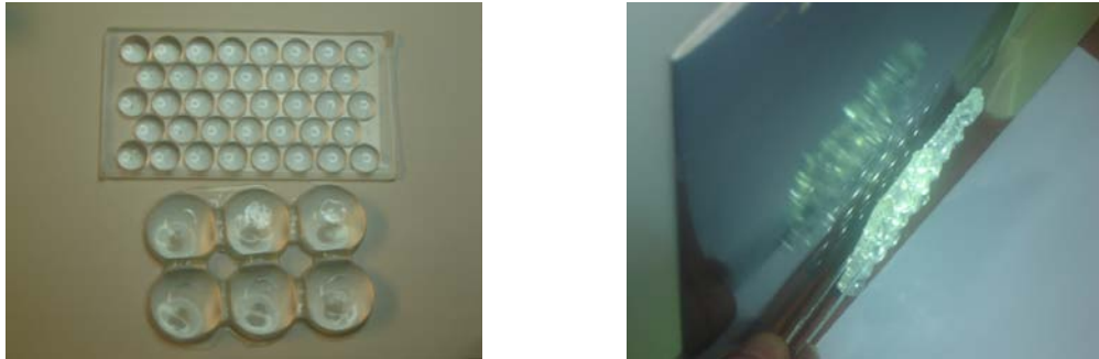
Fig. 7. Various configurations of concentrating systems with small focal length fabricated with PDMS.
