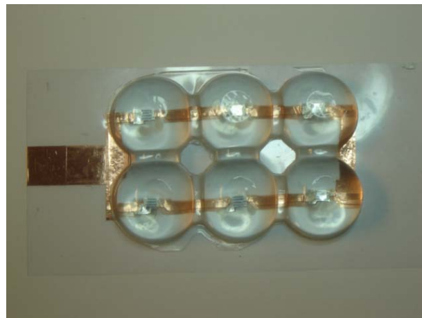
Fig. 8. A solar PV panel containing 6 small area ( 0,5 \text{ cm}^2 ) Si PV cells operating under illumination of 20 suns.
