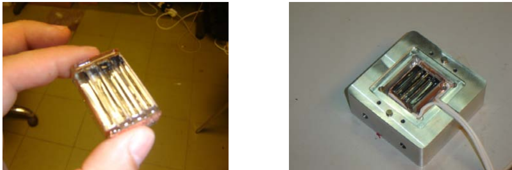
Fig. 6. The FOCUS prototype just packed (left) and before positioning on the optical system for solar light concentration (right).
