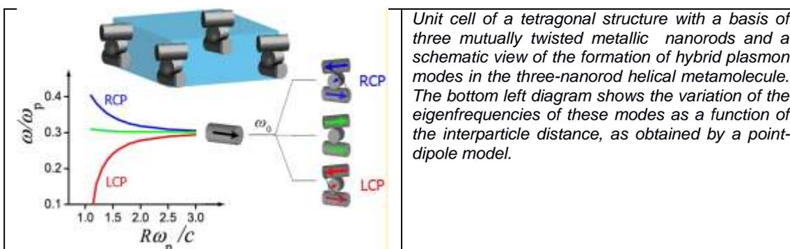
Unit cell of a tetragonal structure with a basis of three mutually twisted metallic nanorods and a schematic view of the formation of hybrid plasmon modes in the three-nanorod helical metamolecule. The bottom left diagram shows the variation of the eigenfrequencies of these modes as a function of the interparticle distance, as obtained by a point-dipole model.
