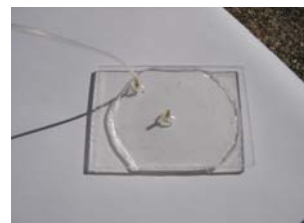
Fig. I.2.6: Chromatography microcolumn fabricated in PDMS with soft lithography and irreversibly bonded on spin-coated PDMS spin-film, well-adhered on a PMMA plate used for mechanical support of the fluidic interconnects
