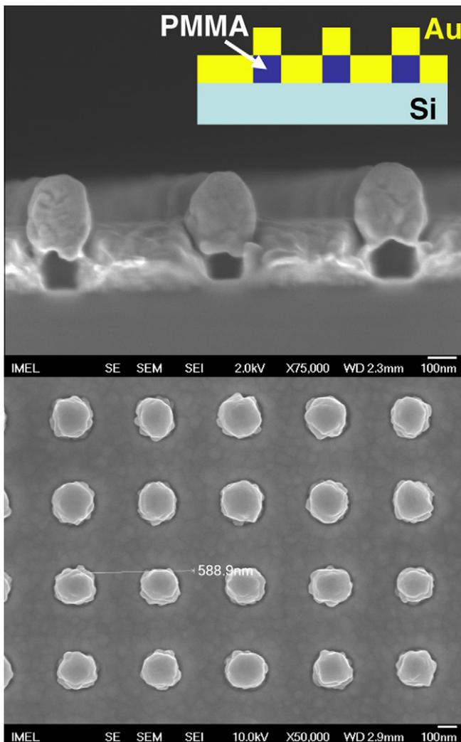
Fig. 1. Typical SEM micrographs of the patterned PMMA after sputtering with Au top: cross section and bottom: top view. In the inset, we show a schematic of the cross-section with the PMMA pillars and the Au film on top.
