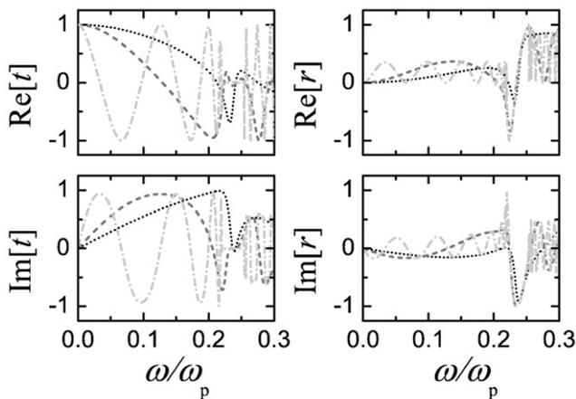
Fig. 3. Complex  $S$ -matrix parameters of one- (dotted lines), two- (dashed lines) and eight- (dash-dotted lines) layers thick (001) slabs of the crystal under consideration (neglecting absorptive losses), at normal incidence.
